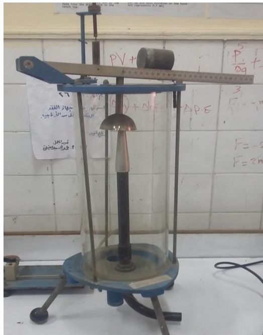
Impact of water jet on flat and hemispherical plate
