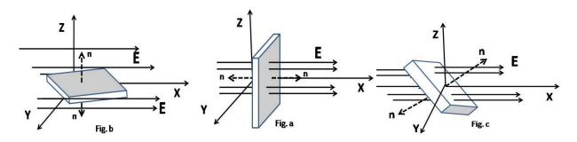
Electric flux  $\varphi$  is determined by knowing the electric field E and the perpendicular area A<sub>n</sub> where
